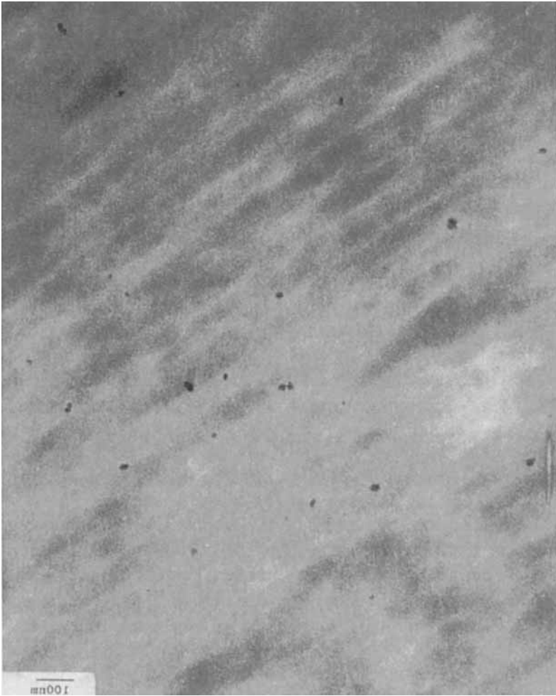
FIGURE 3 Transmission electron micrograph through microtomed injection molded PET containing elemental antimony particles of 10–25 nm size, created in-situ by the reduction of antimony-catalyst residues. Original magnification: 70,000 x.
